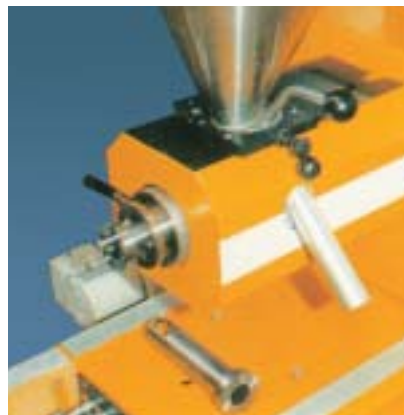
Divided barrel with interchangeable grooved bush
