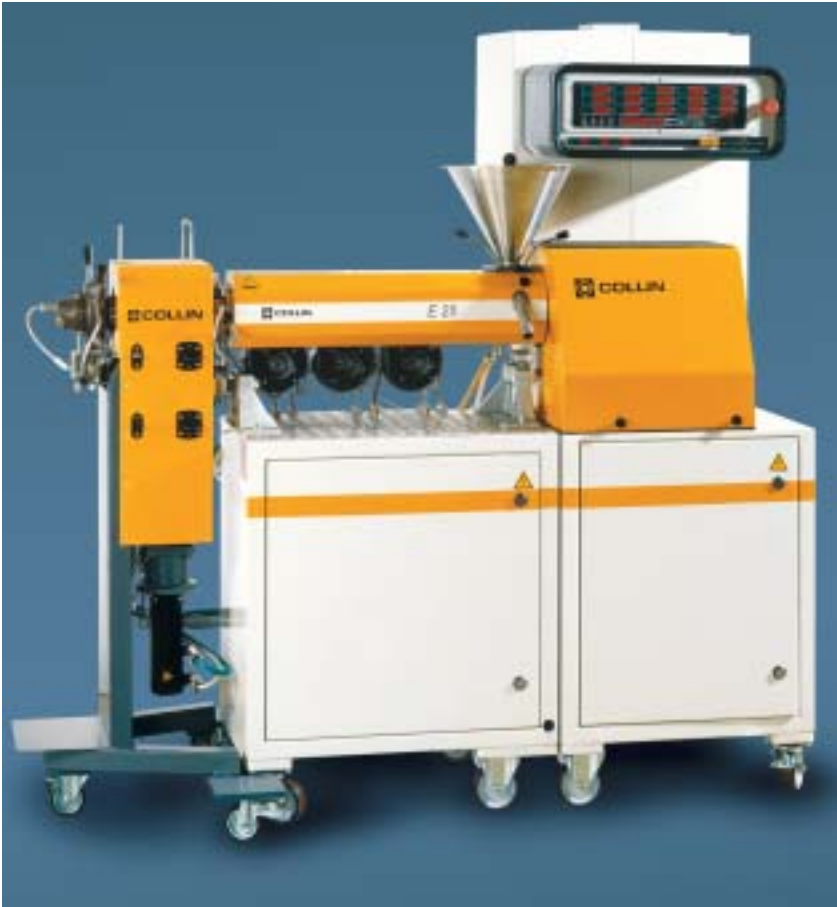
Extruder 25 mm Ø with melt pump for the pressure filter test
