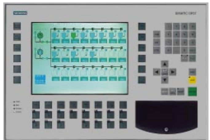
Process visualisation by means of a control unit MST-24/PDP
