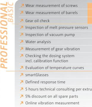
We recommend the first check up 10-12 months after commissioning, then annually. \*Option: permanent online vibration control of all gearbox and main motor bearings.
