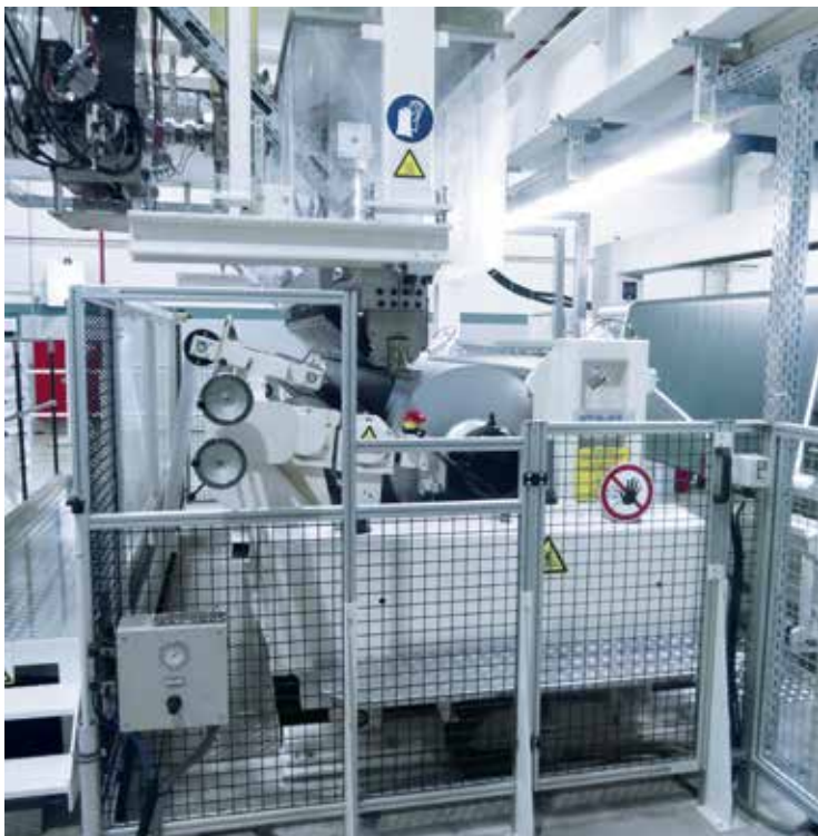
integrated laminator for spunbond line
