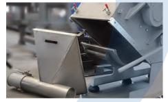
The user friendly design of the GSE series granulators allows quick and easy access to the cutting chamber for maintenance and cleaning.
