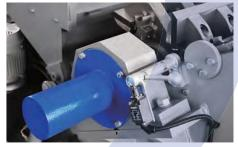
The heavy duty bearings are separated from the cutting chamber to avoid lubricants entering the cutting chamber and bearing failure due to material contamination in the bearings.
