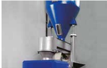
The material is fed into the Pulverizer by a vibrating dosing channel, the feeding rate is automatically adjusted based on the motors amperage and material temperature.
